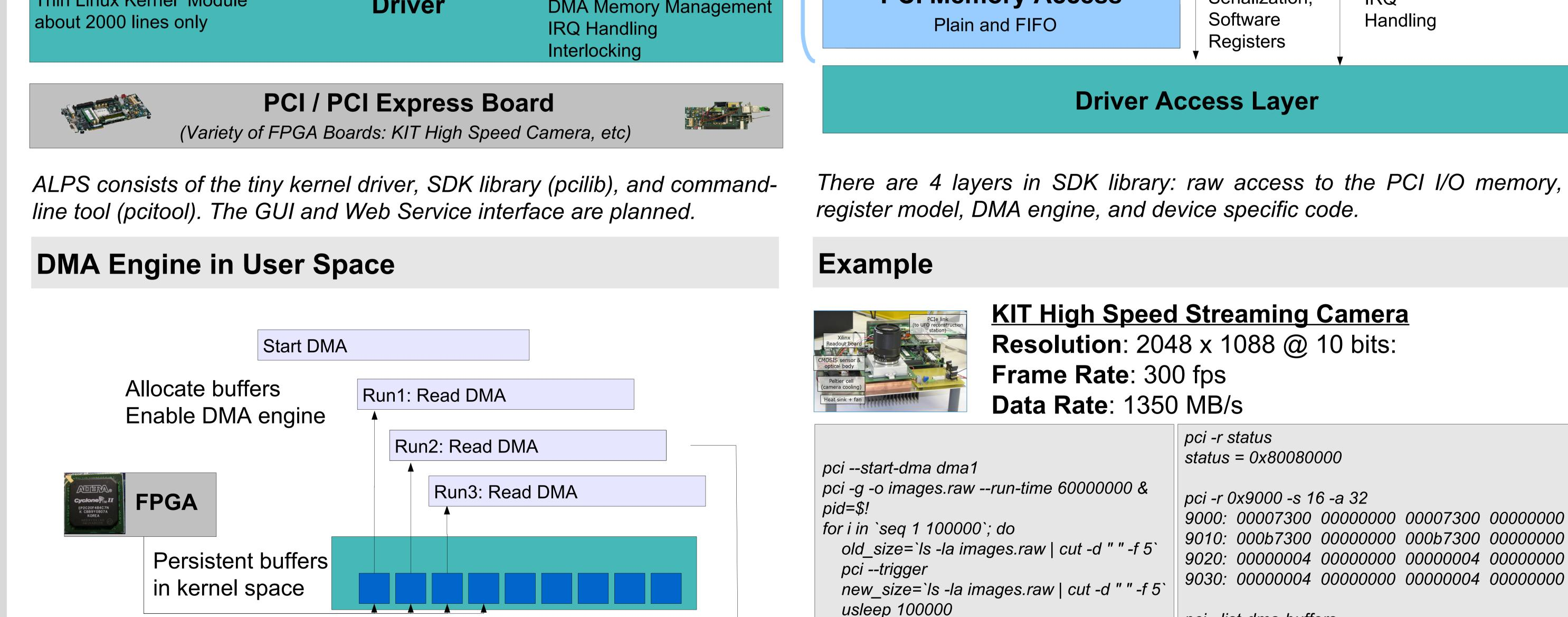
**Reusing buffers** •Check if buffer already allocated •Positionate reading pointer •Get Data •Mark buffer free & ready
