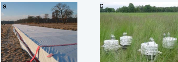
Fig. 1: The tunnel (a) with its dimensions and the FTIR unit (b), and the closed chambers (c) located at the same plot.
