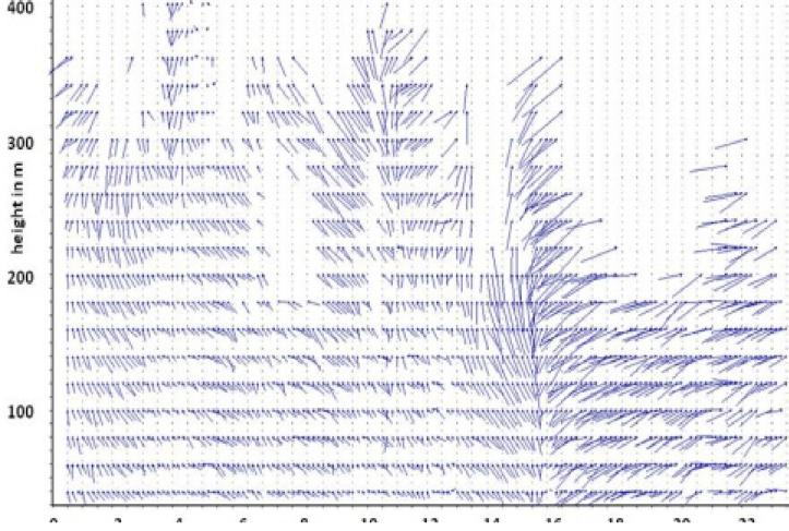
Active acoustic plus electromagnetic sounding with a SODAR-RASS delivers vertical wind, turbulence and temperature profiles and mixing-layer height up to about 600 m (10 to 20 m vertical resolution)
