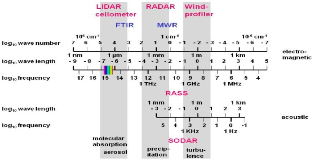
Active acoustic sounding with a Doppler-SODAR delivers vertical wind and turbulence profiles and mixing-layer height up to about 1000 m (10 to 20 m vertical resolution)
