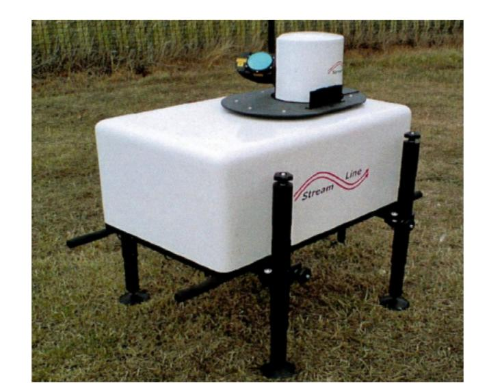
Active optical sounding with a small Doppler-LIDAR delivers vertical wind, turbulence and aerosol profiles and mixing-layer height up to several 1000 m (10 to 20 m vertical resolution) sounding result: diurnal variation of horizontal wind velocity (m s<sup>-1</sup>) in the atmospheric boundary layer from June 22<sup>nd</sup>, 2011 in Garmisch-Partenkirchen.
