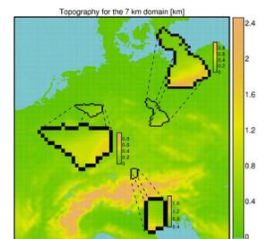
Figure 2: RCM Domain 2 (7km) and river catchments under study: Ammer (south), Mulde (east) and Ruhr (west)
