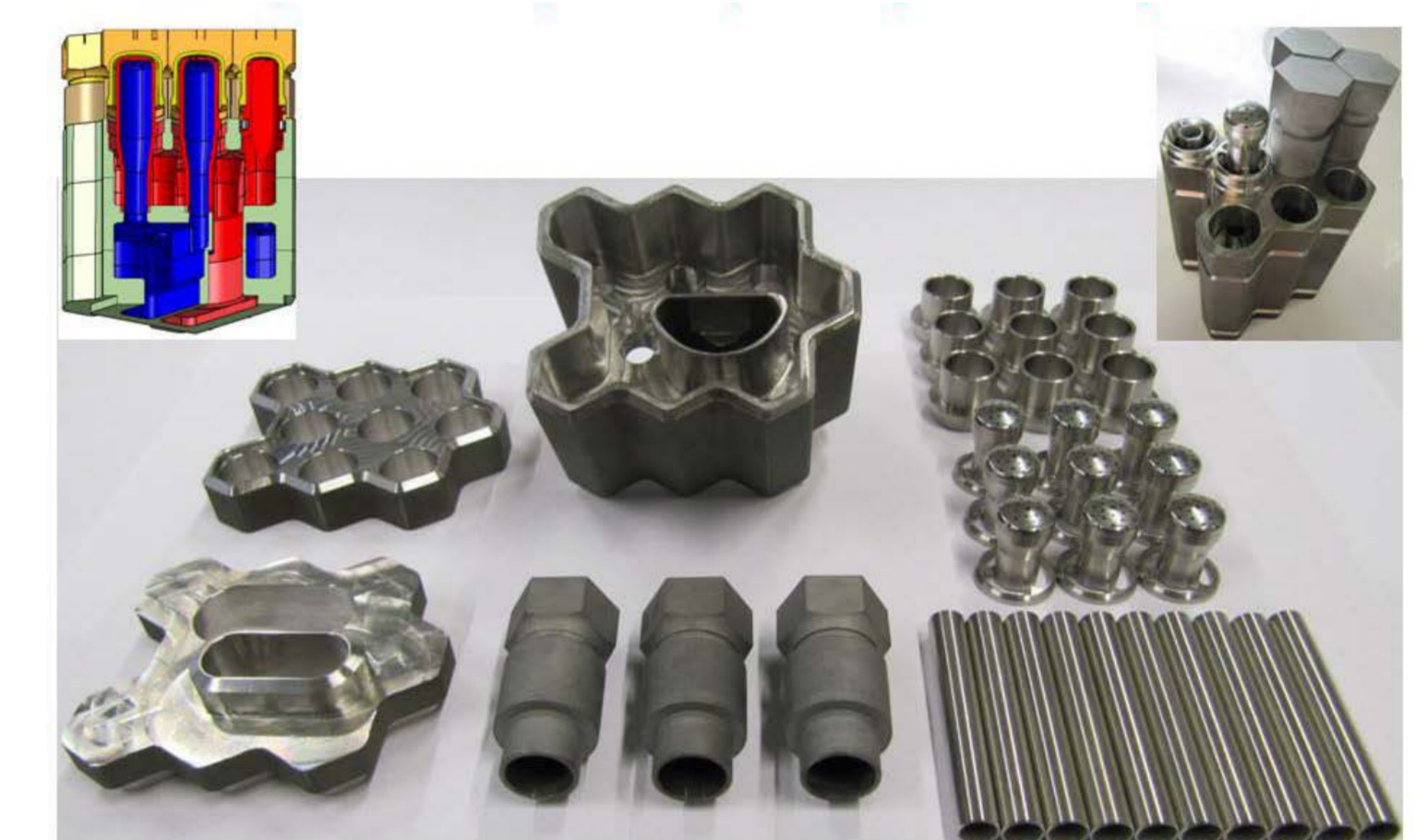
Manufacturing of the 9-finger module for the Helium cooled divertor developed in KIT. In 2010 a new series of tests conducted at the Electron Beam facility in Efremov achieved a first breakthrough in the qualification programme for such as divertor target: one finger was able to survive 1000 cycles at 10 MW/m 2 under high temperature helium cooling.
