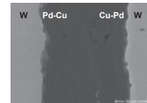
Pd-Cu layers on W after annealing at 1100°C / 10 min.
