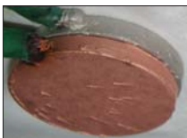
W discs plated by Pd and Pd and Cu layers
