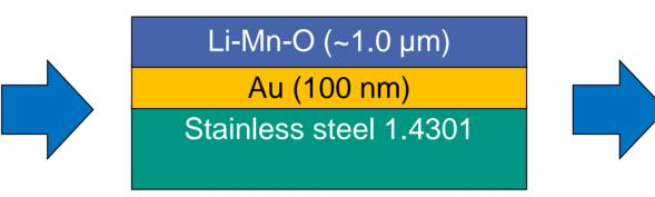
It was possible to synthesize three different cathode materials, which are of potential interest in future thin film lithium ion battery applications.
