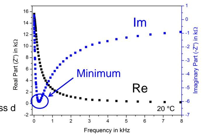
In the case of a system with a capacity like behavior, the imaginary part has a minimum in the frequency range between 10 Hz and 1 MHz. This leads to a semicircle in the Nyquist diagram.
