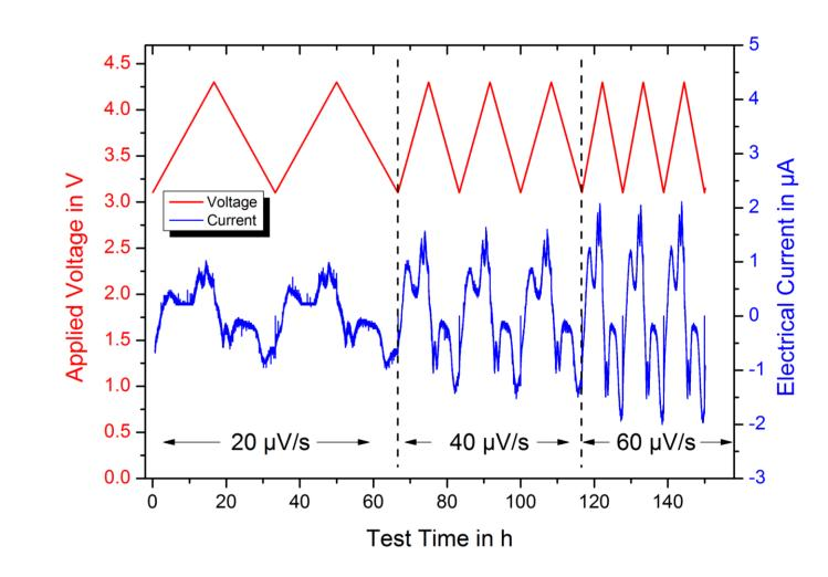
During the measurement a triangle shaped voltage ramp is applied to the cell. The current is measured simultaneously.
