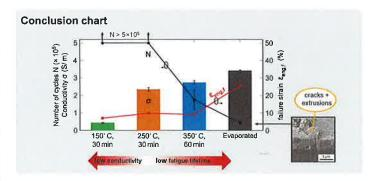
A nanoparticle silver ink was printed on polyimide substrates and annealed at different temperatures.
