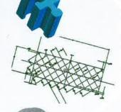
**LIGA2.X** a modified LIGA process sequence for the fabrication of polymeric single micro parts
