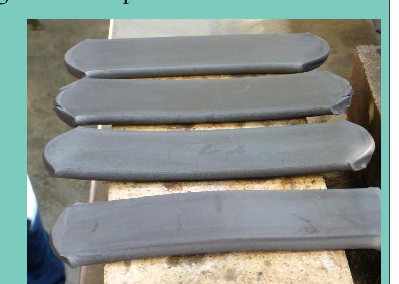
A final heat treatment was performed at 800°C for 1 hour.
