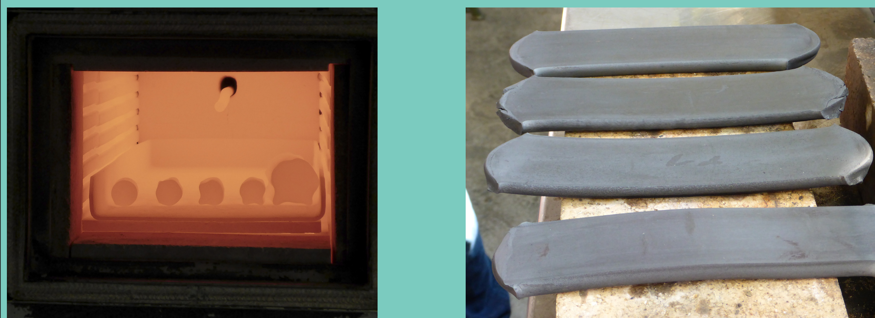
A final heat treatment was performed at 800°C for 1 hour.
