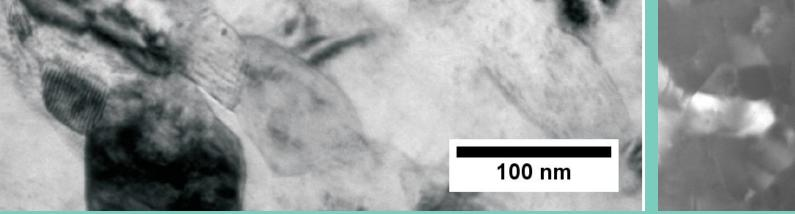
Small nanometer oxide clusters in the range between 10-15 nm could be observed in TEM images.
