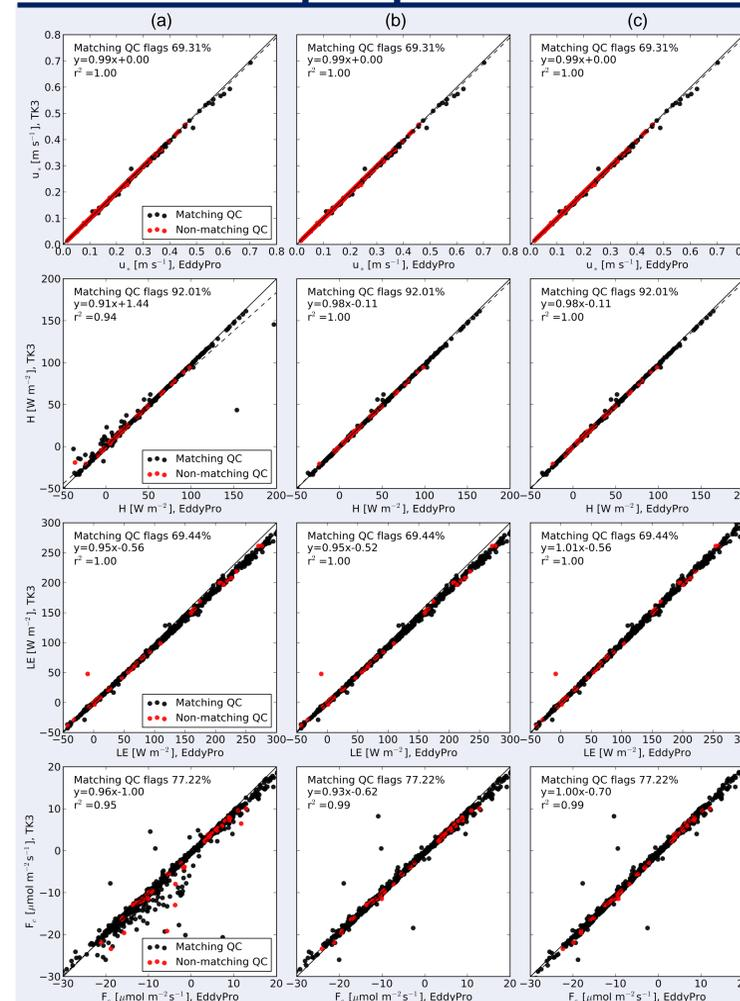
(a) The scatter observed in the first round is due to using or not the pressure data available among the raw data. Significant systematic differences is observed for both  $F_c$  and LE.
