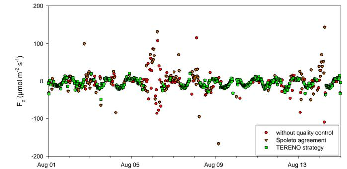
Figure 2: CO<sub>2</sub>-fluxes for Graswang: without quality control (red circles), flagging according to FW96/Spoleto (orange triangles), filtering according to TERENO quality assessment scheme (green squares)
