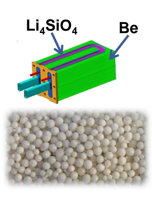
Due to the nature of the melt based process used at KIT, it is proposed that the depleted pebbles can be reenriched with lithium by remelting them in the standard process crucible with additions of LiOH. In order for this method to be considered as a suitable reprocessing route, as opposed to wet chemical processing, it is necessary to demonstrate the feasibility of both recycling the material, as well as replenishing the <sup>6</sup>Li after burnup, whilst minimising impurities.
