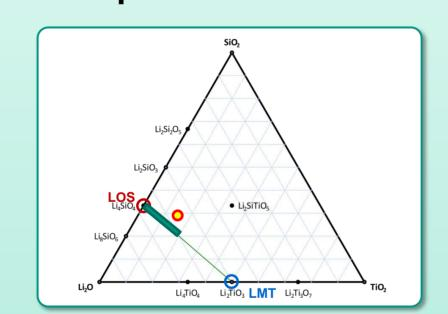
The pebbles were remelted with corresponding quantities of LiOH to gain the intended composition of the starting material.
