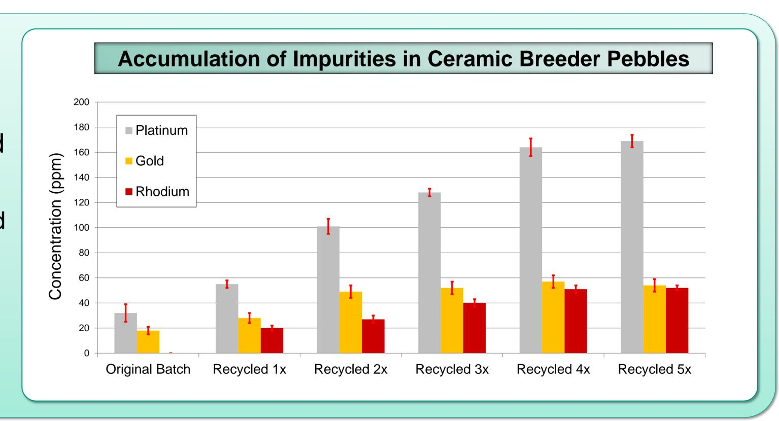
Pebbles were produced that represented a burn-up of 15% with an enrichment of 50% <sup>6</sup>Li (expected to occur during the lifetime in the reactor wall) resulting in pebbles with the following composition:
