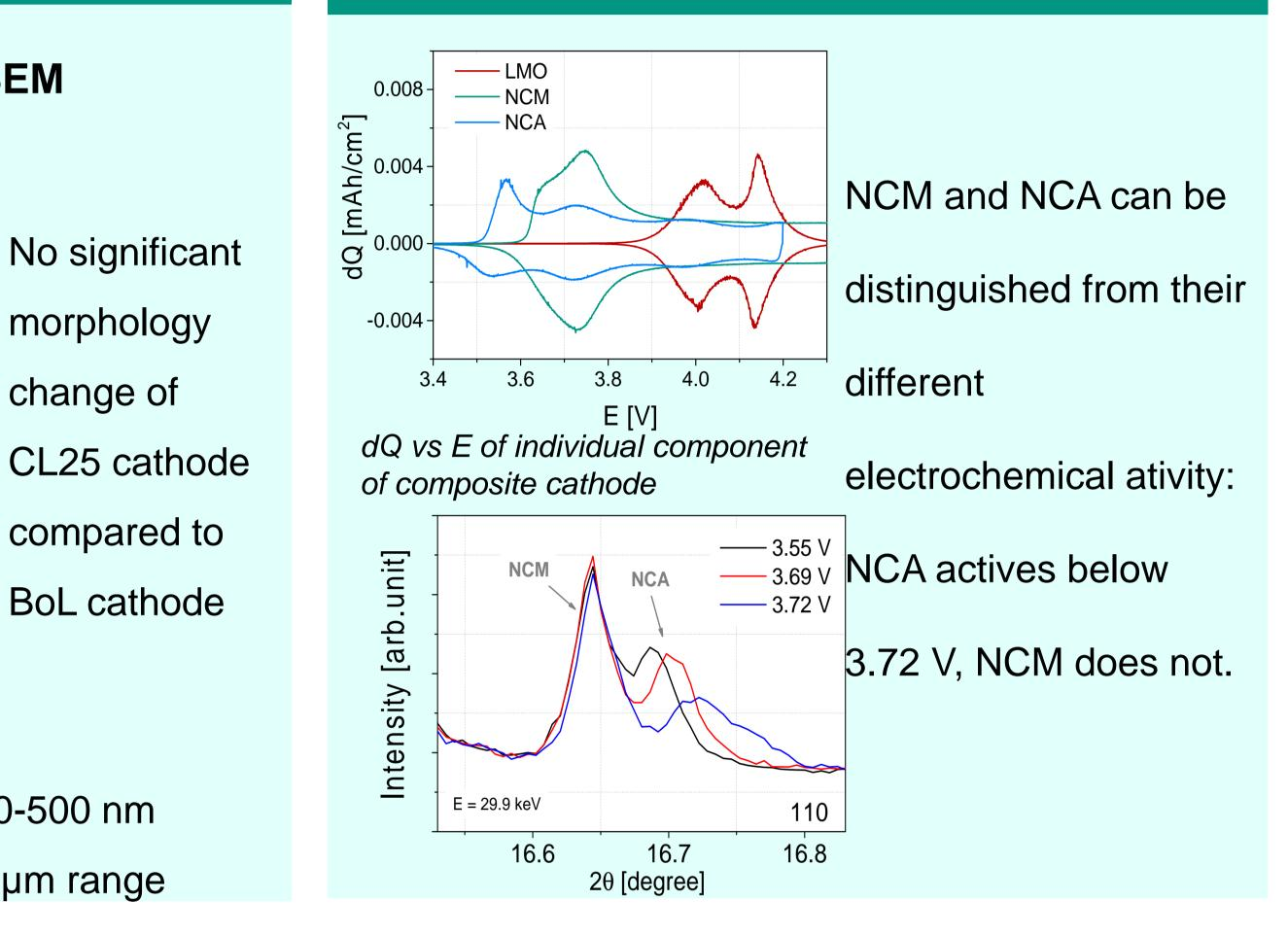
**Specific Phase Degradation at Room Temperature by in situ XRD**
