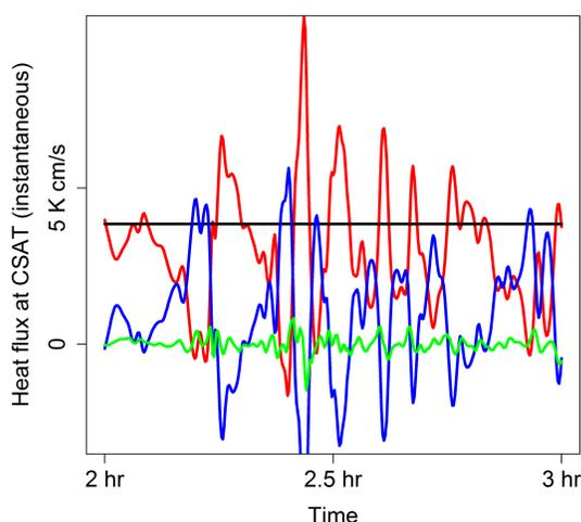
Fluctuations of the instantaneous virtual heat flux at the measurement height (red). The available energy (black) is taken as the surface heat flux. The storage term (blue) matters due to the significant measurement height. The model non-conservation residual (green) is close to zero but fluctuates more strongly if the area of the control volume is smaller.
