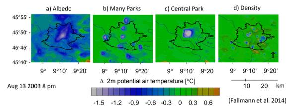
Fig. 4: Difference in potential 2m air temperature between 'Control' and 'Scenario'
