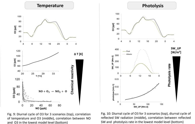
Fig. 9: Diurnal cycle of O<sub>3</sub> for 3 scenarios (top), correlation of temperature and O<sub>3</sub> (middle), correlation between NO and O<sub>3</sub> in the lowest model level (bottom)
