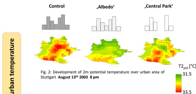
Fig. 2: Development of 2m potential temperature over urban area of Stuttgart August 13th 2003 8 pm
