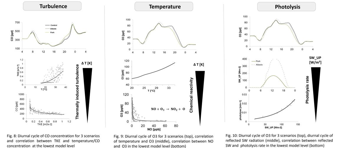
Fig. 8: Diurnal cycle of CO concentration for 3 scenarios and correlation between TKE and temperature/CO concentration at the lowest model level
