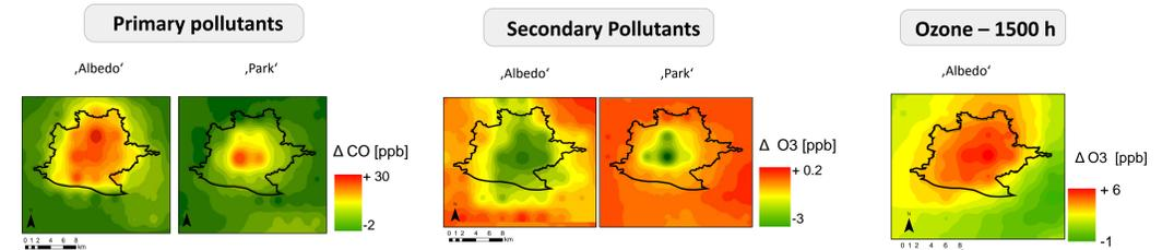
Fig. 7: Mean Difference between control- and scenario run [ppb] for modelling period for carbon monoxide (left), ozone (middle) and difference in peak ozone concentration at 1500 h (right)
