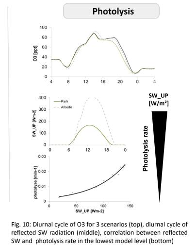
Fig. 10: Diurnal cycle of O<sub>3</sub> for 3 scenarios (top), diurnal cycle of reflected SW radiation (middle), correlation between reflected SW and photolysis rate in the lowest model level (bottom)
