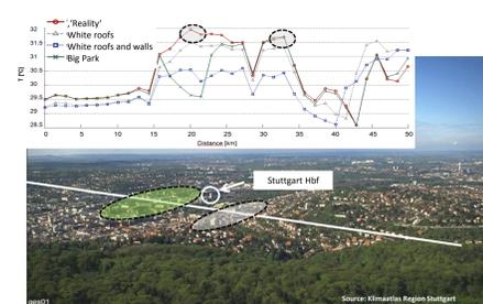
Fig. 3: Development of 2m potential temperature over cross section (left) and for the urban area of Stuttgart (right) August 13th 2003 8 pm
