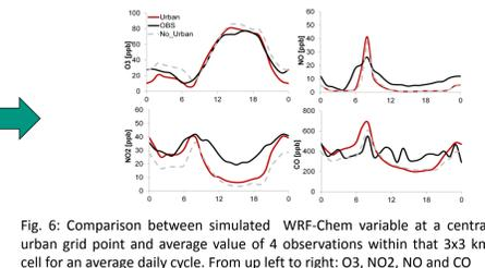
Fig. 6: Comparison between simulated WRF-Chem variable at a central urban grid point and average value of 4 observations within that 3x3 km cell for an average daily cycle. From up left to right: O<sub>3</sub>, NO<sub>2</sub>, NO and CO
