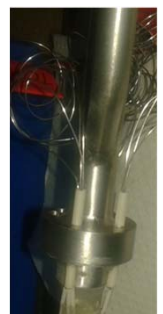
Thermocouple feedthrough of AMTEC cell
