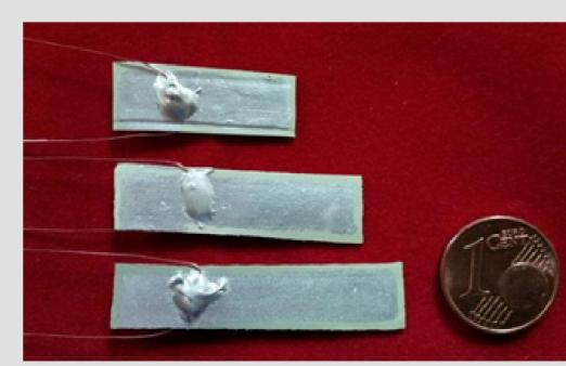
**Piezoelectric triplelayer bending transducers** with interdigital Ag electrode structure fabricated by casting both ceramic and metallic layers. After co-firing and applying outer electrodes, the MLs were poled in silicon oil. Wire bonding was made provisionally with conductive epoxide glue.
