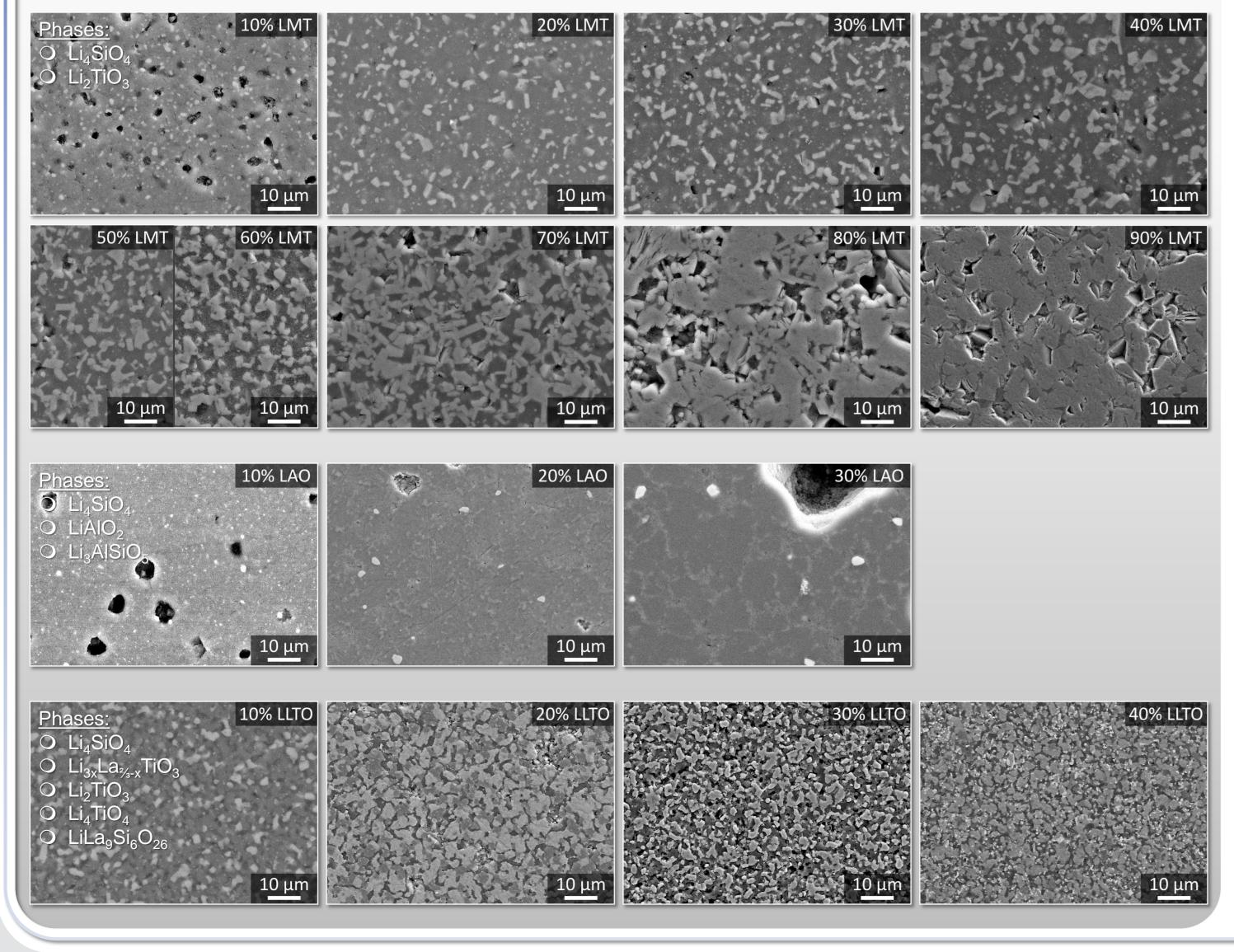
The microstructure is in general very homogenous with reasonably small grains. The addition of one of the tested second phases to the LOS pebbles increases the pebble rigidity. LLTO reacts with LOS, yet, the product excels in mechanical strength. According to the observed phases, LOS+LAO samples show a mild loss of lithium.
