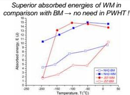
Motivation: A potential needlessness in PWHT of EB welds does not exclude the necessity to study the effect of post-weld heating to working temperatures on the mechanical and structural properties of weld zones!
