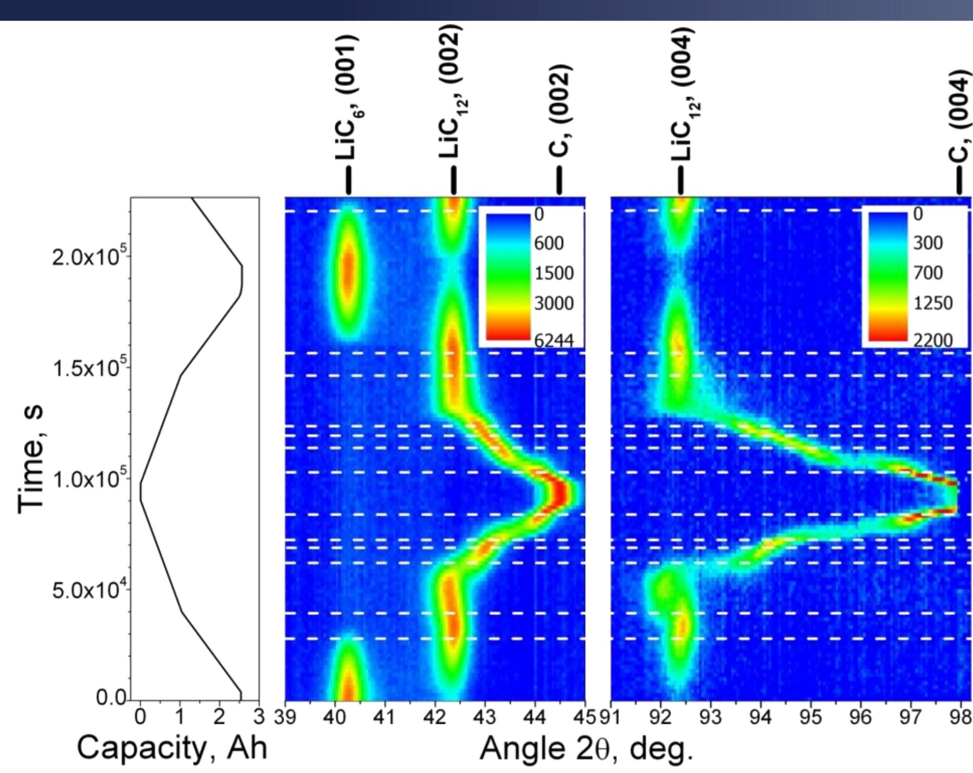
Time resolved neutron diffraction revealing an asymmetry in lithium intercalation
