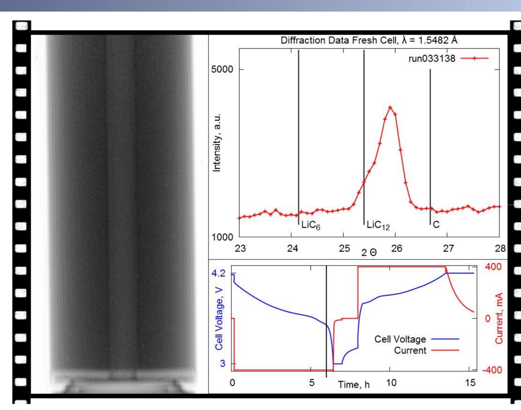
Charge and discharge of cells with simultaneous acquisition of neutron diffraction and imaging data
