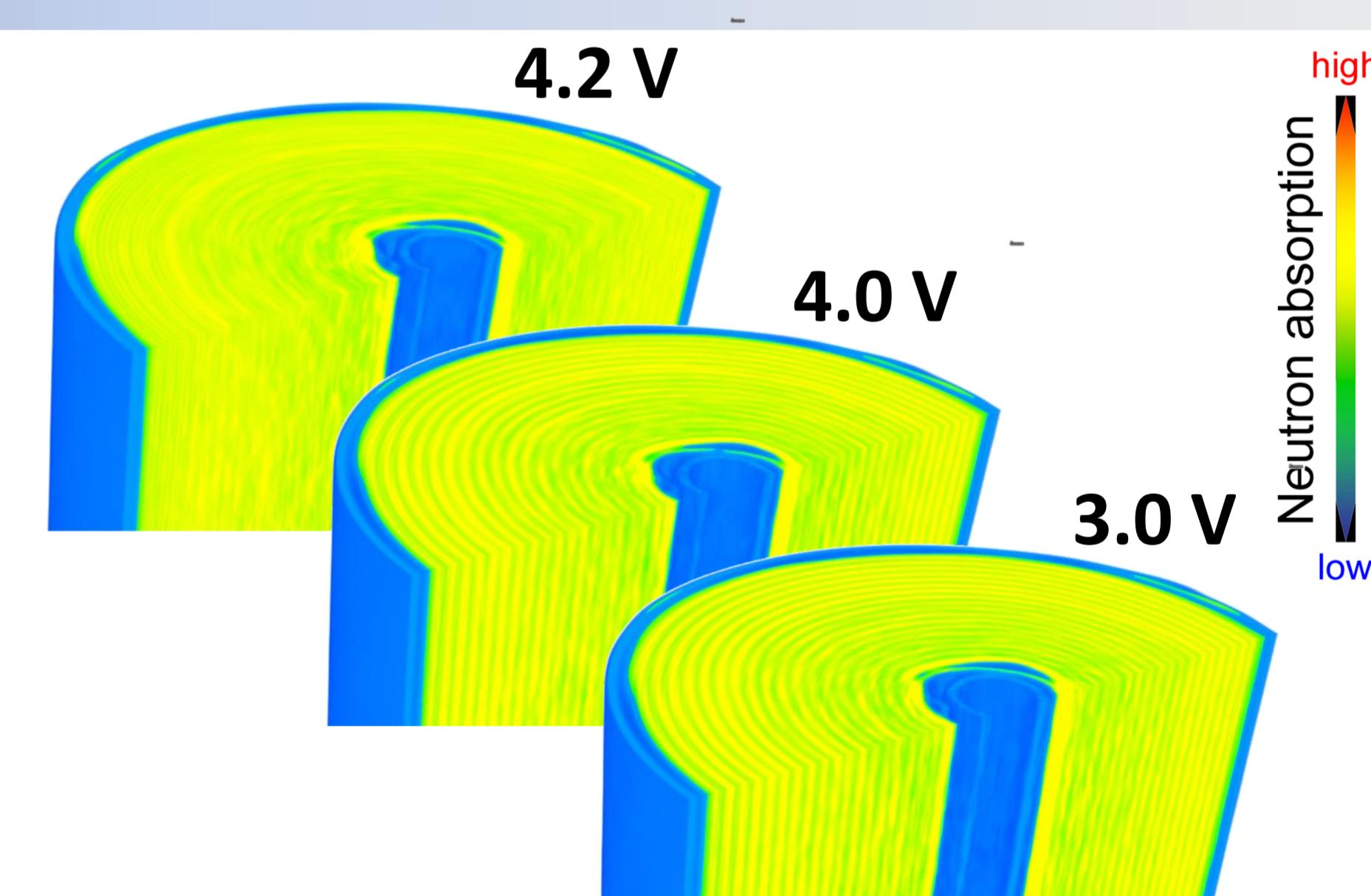
Exchange of lithium causes the neutron attenuation to change according to the state of charge
