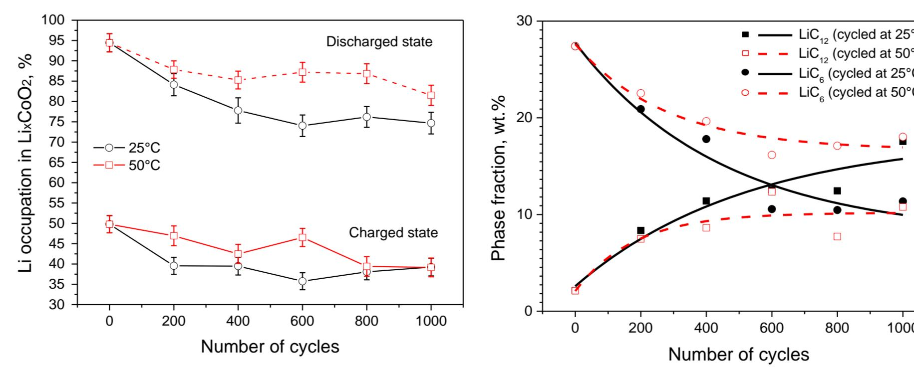
Lithium occupation of cathode and anode for different states of fatigue
