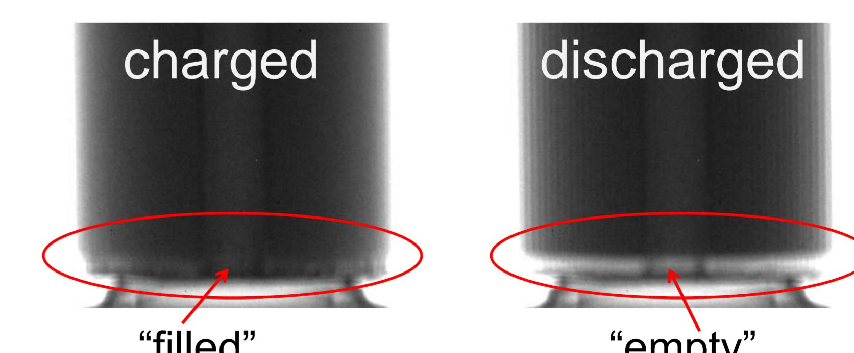
Due to volume change of the electrodes the electrolyte level inside the reservoir is altered
