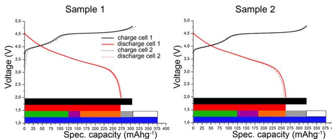
The value for theoretical charge capacity is related to overall amount of Li ions. The theoretical capacity for NCM is based on accessible oxidation states of Ni and Co. The capacity contributions were calculated using the presented mechanism.
