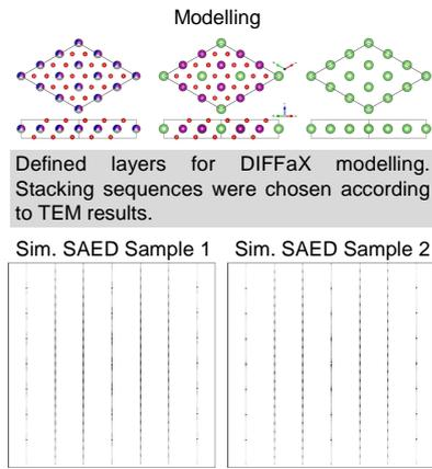
DIFFaX is used to estimate  $\text{Li}_2\text{MnO}_3$  domain thickness and diameter by implementing defect free  $\text{Li}_2\text{MnO}_3$  stacking sequences in randomly stacked  $\text{Li}_2\text{MnO}_3$  and NCM layers.
