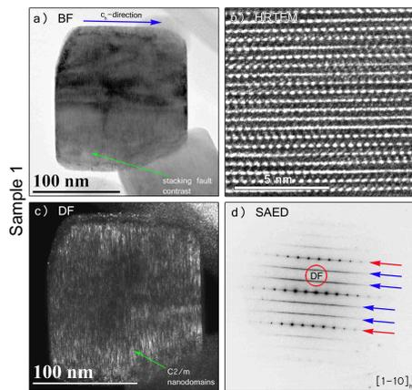
Sample 1: very thin platelet shaped  $\text{Li}_2\text{MnO}_3$  nano domains are evenly dispersed in the particle.
