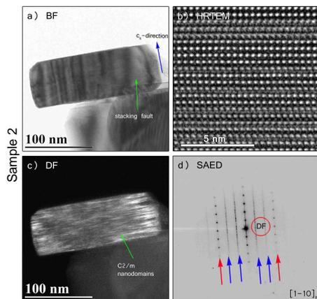
Sample 2: thicker platelet shaped  $\text{Li}_2\text{MnO}_3$  nano domains with larger diameter evenly dispersed in the particle.
