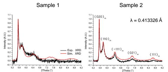
Defect free stacking sequences of 1-5  $\text{Li}_2\text{MnO}_3$  layers and a layer diameter of 100 nm has been used. Defect free stacking sequences of 5-35  $\text{Li}_2\text{MnO}_3$  layers and a layer diameter of 180 nm has been used.
