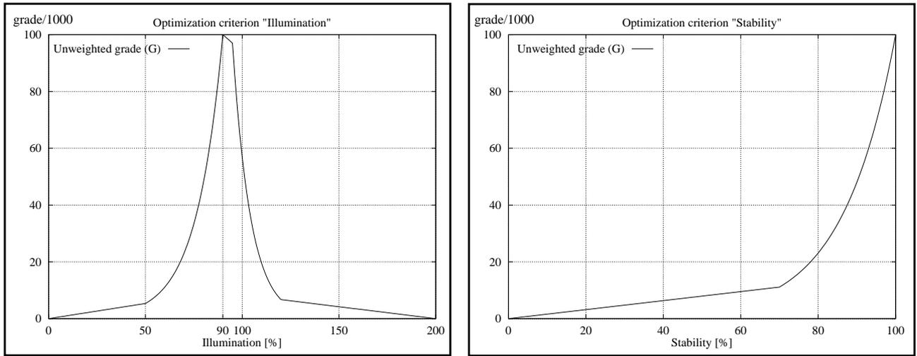
Fig. 3: Grading functions for (left) illumination and (right) stability.
