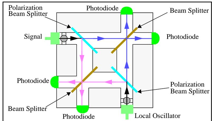
Fig. 5: Scheme of a Heterodyne Receiver
