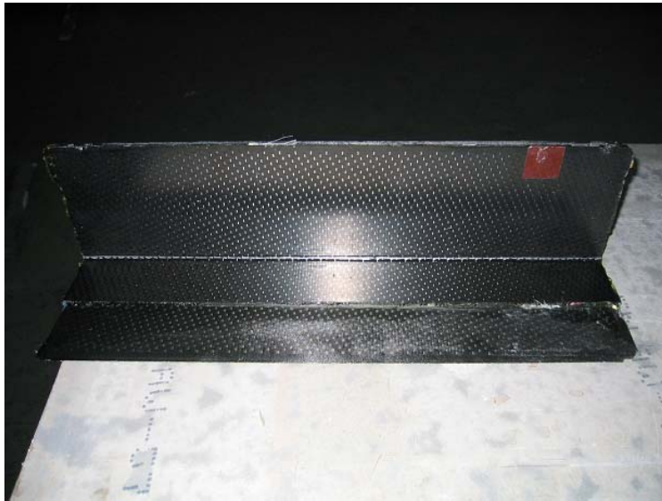
Fig.8: A T-profile fabricated with the HEPHAISTOS-CA1 according the VAP infiltration technology and cured at 180°C
