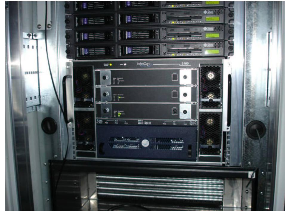
Infinicon 9100, Infiniband switch, MPI latency  $4.0 \mu\text{s}$  between nodes
