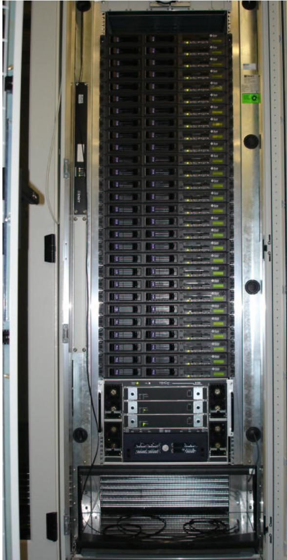
watercooled Infiniband cluster with 32 SUN V20z and 32 FSC RX220 nodes
