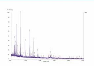
Fig. 4: MS-spectrum of trypsin-digested penicillin G acylase (MALDI-TOF/TOF)
