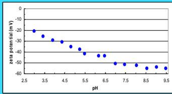
Fig. 3: Zeta potential of the silica nanobeads
