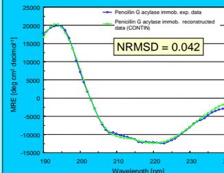
Fig. 7: Comparison of experimental and reconstructed spectrum of the immobilized enzyme (CONTIN algorithm)
