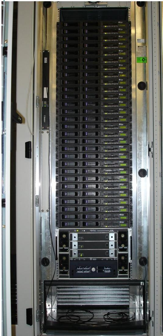
watercooled Infiniband cluster with 32 SUN V20z and 64 FSC RX220 nodes (more than 190 cores and >1 TByte main memory)
