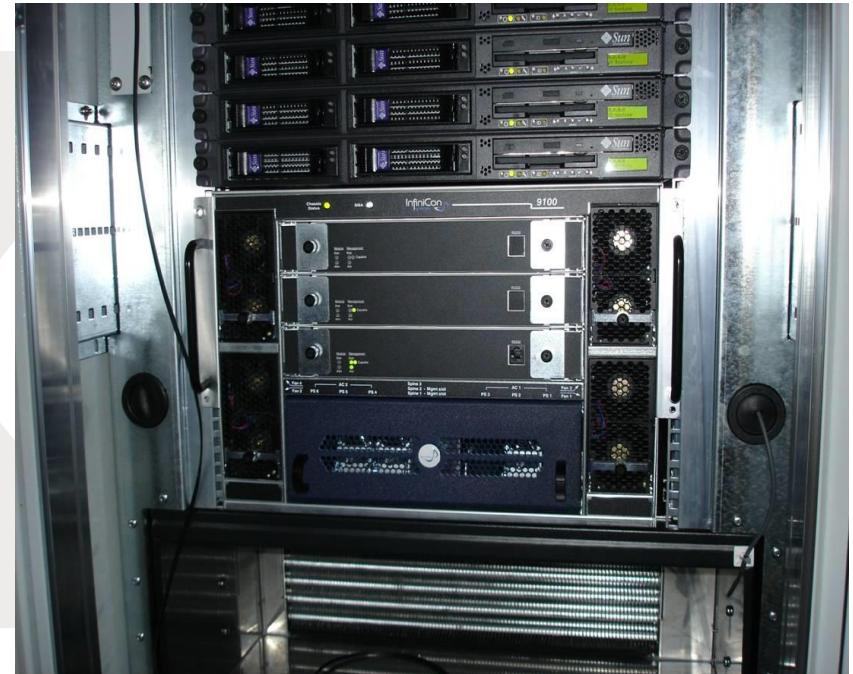
2 Infinicon 9100, Infiniband switches, MPI latency 4.0  $\mu$ s between nodes
