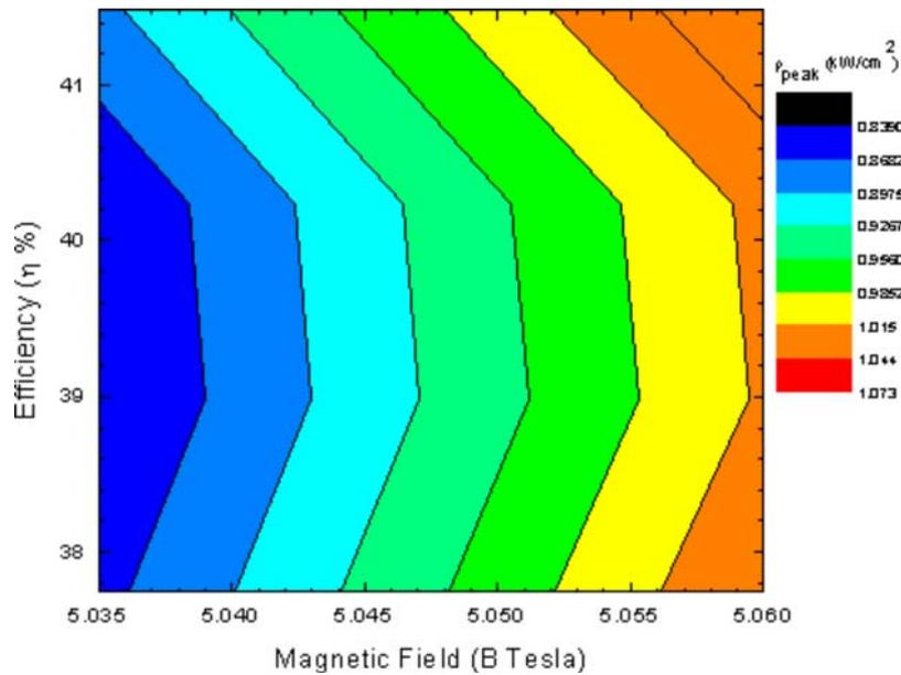
Fig. 3 Random contours of peak wall loading for a TE<sub>24,8</sub> mode gyrotron.
