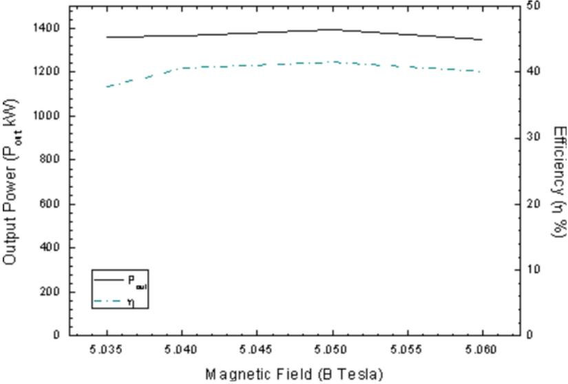
Fig. 2 Self-consistent simulation results for a  $TE_{24,8}$  mode gyrotron.
