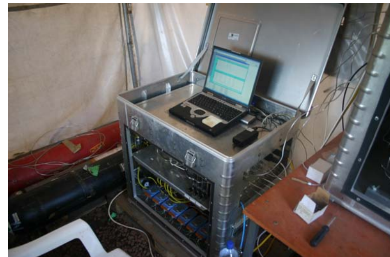
On-line GC analysis in the field
