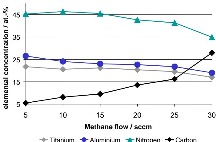
Characterisation method: electron probe micro analysis (Cameca microbeam system)
