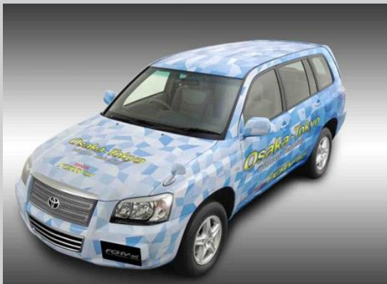
Toyota FCHV 70 MPa 90 kW PEM fuel cell stack, hybrid with Ni MH battery; range 560 km
