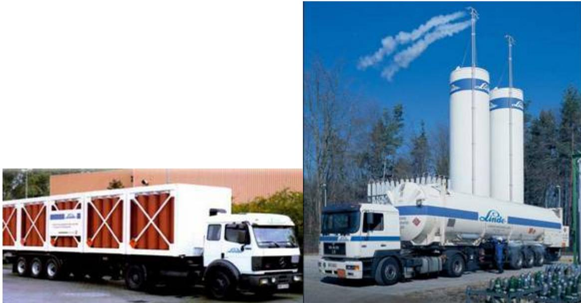
Figure 37: CGH2-Truck (40t total weight) with 530 kg CGH2 and LH2-Truck with 3370 kg LH2 (less than 40t total weight)
