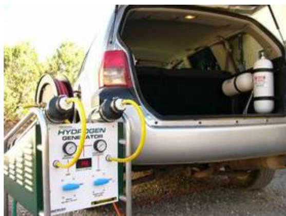
Figure 59: Mitsubishi Endeavour equipped with additional  $CGH_2$  pressure vessels; small electrolyser for home refuelling in the front [[www.switch2hydrogen.com/h2.htm](http://www.switch2hydrogen.com/h2.htm)]
