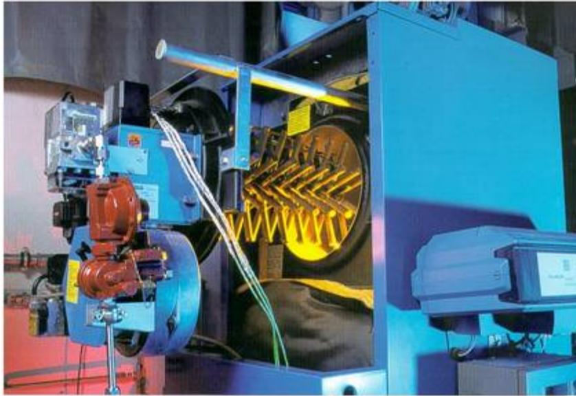
Figure 55: Catalytic H2 Burner [25]
