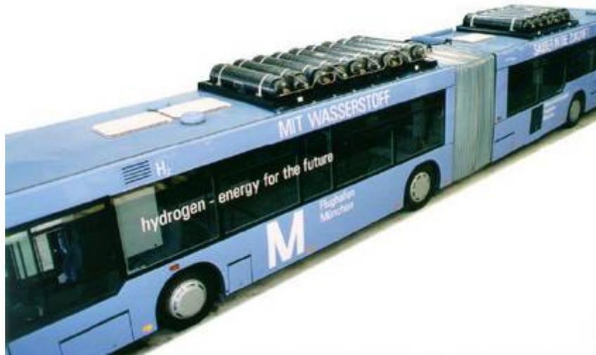
Figure 30: Dynetek CGH2 Storage for the MAN Buses at the Munich Airport.
