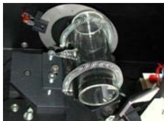
Fig. 2. Low density HCl cell to monitor the instrumental line shape.
