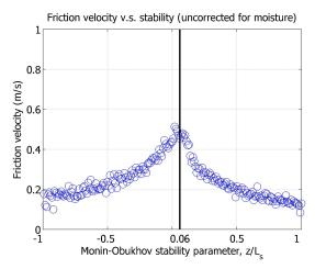
Stability is over predicted since the peak friction velocity is detected on the slightly stable side if the stability parameter is not corrected for humidity effects (Here, <sup>z</sup>/<sub>Ls</sub> = <sup>zkg ≤ wT<sub>s</sub>≥).</sup>
