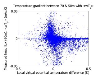
Local heat fluxes are poorly correlated with local temperature gradients. (Correlation coefficient: -0.06)
