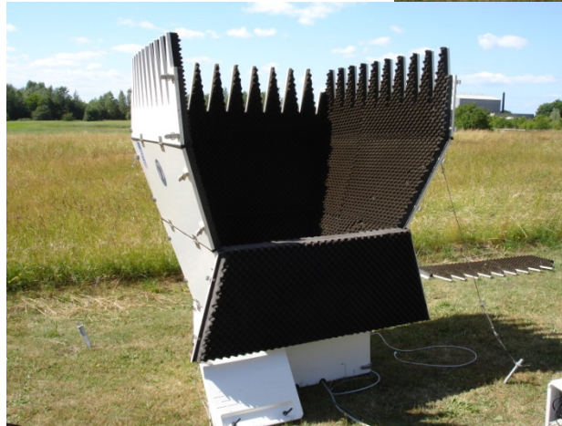
phased-array SODAR range: roughly 600 m
