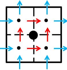
**STEP 1**: Coarse grid velocity (divergence free) → external fine grid velocites
