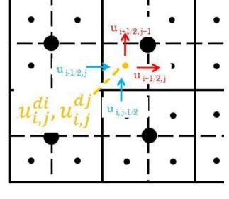
Interpolation of the velocity gradient
