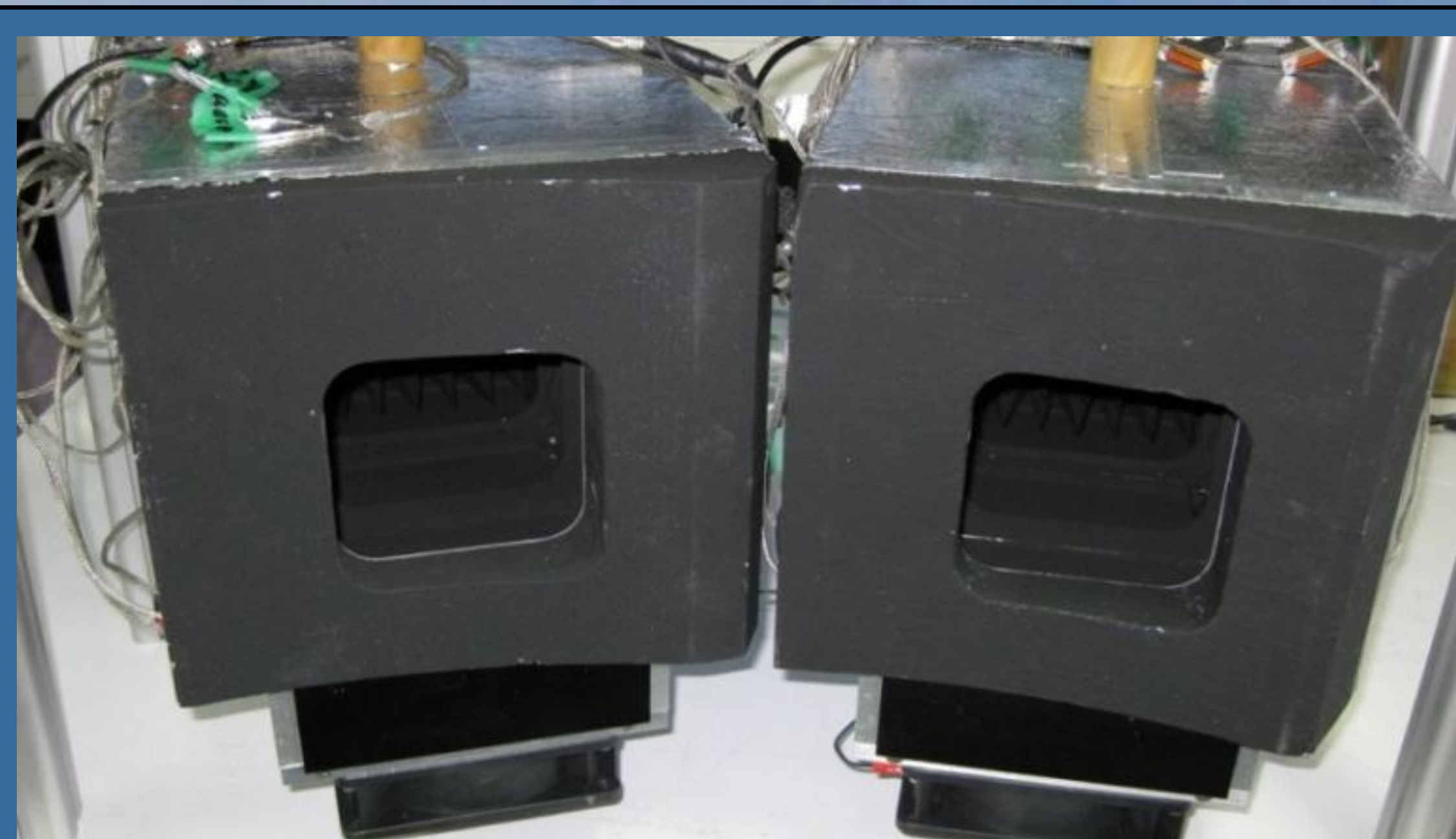
Figure 2: GLORIA In-flight Calibration System
