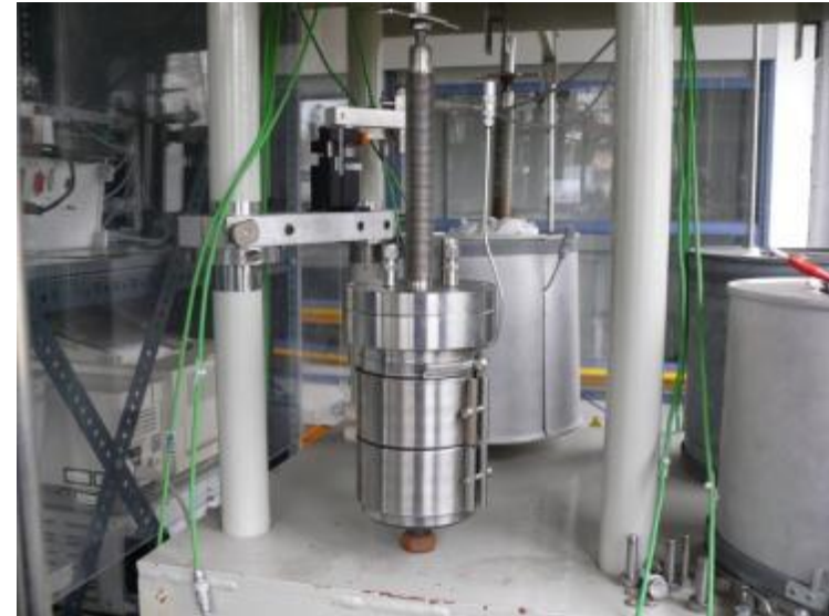
Displacement transducer outside the capsule
