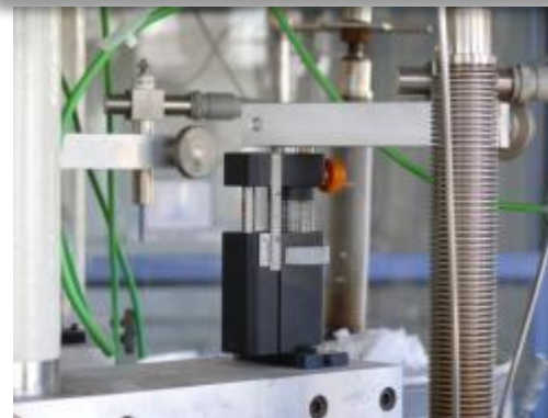
Displacement transducer outside the capsule
