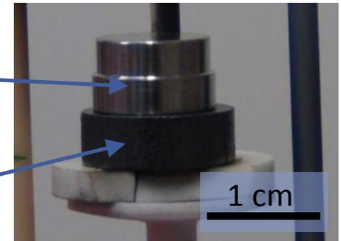
➡ **Rapid and complete melting of SS at 1250°C starting at  $B_4C$ /SS boundary**
