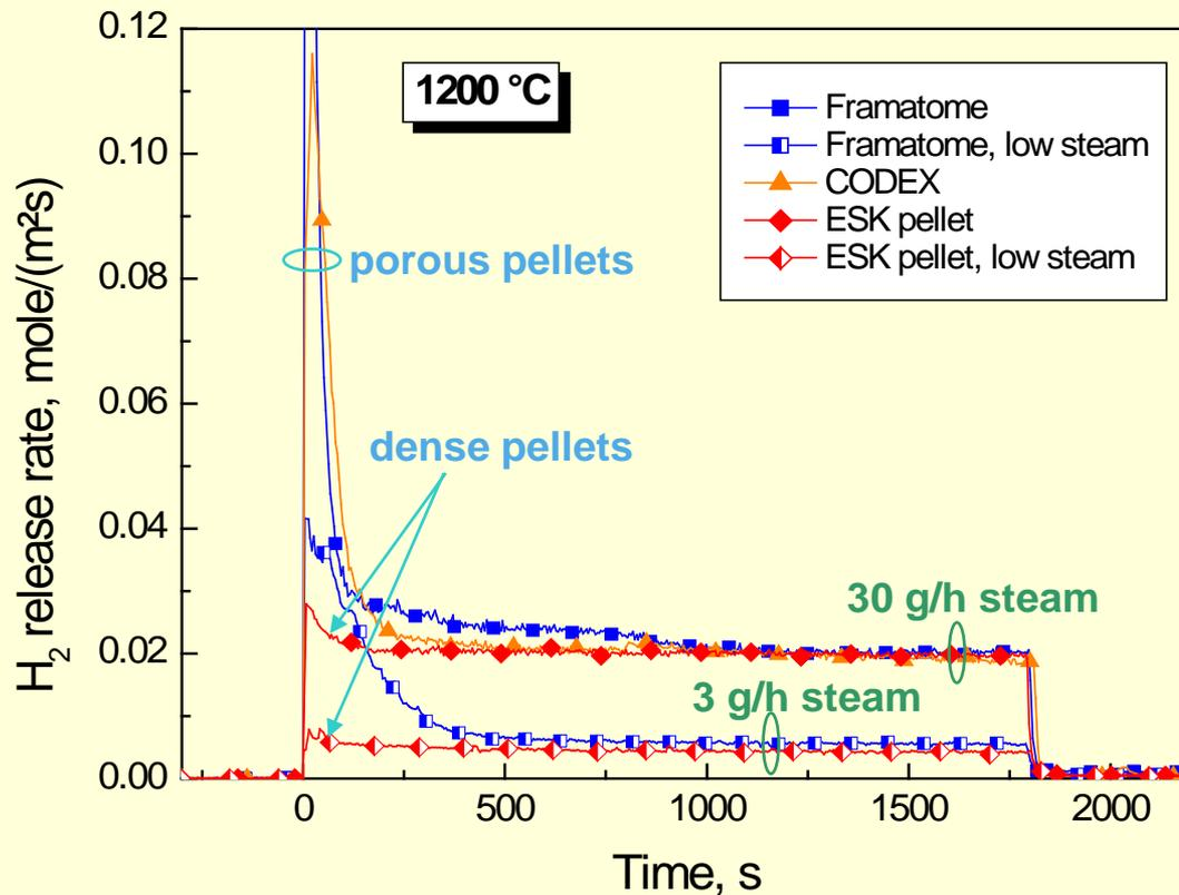
Strongly dependant on B<sub>4</sub>C structure and thermo hydraulic boundary conditions like pressure and flow rate
