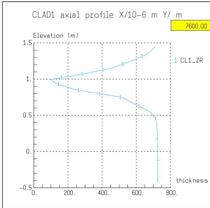
Fig.8 Oxide thickness profile, 7600 s, unheated rod - ASTEC
