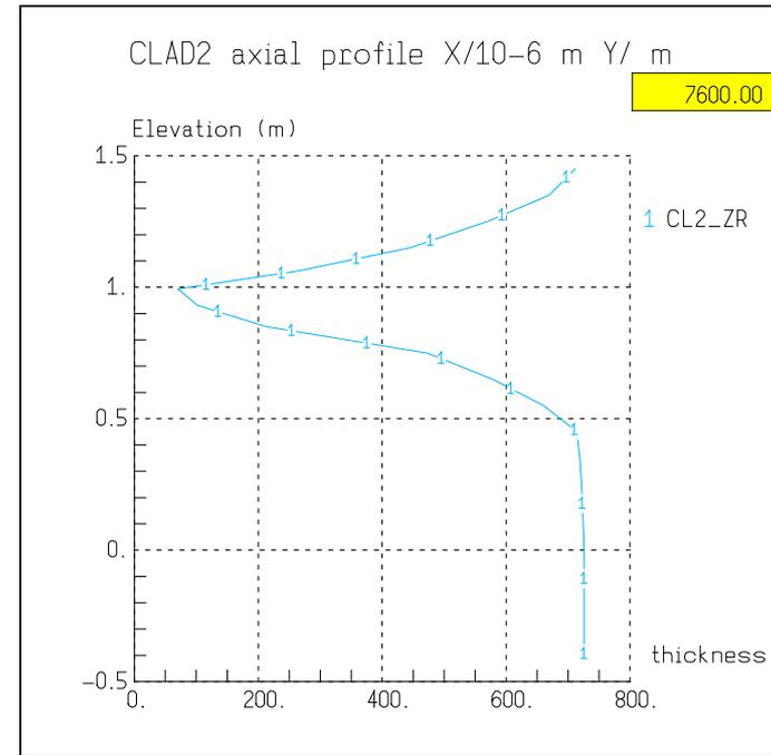
Fig.9 Oxide thickness profile, 7600 s, inner ring rod, 7600 s - ASTEC
