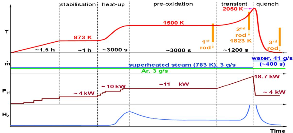
Fig.3 QUENCH-14 test phases
