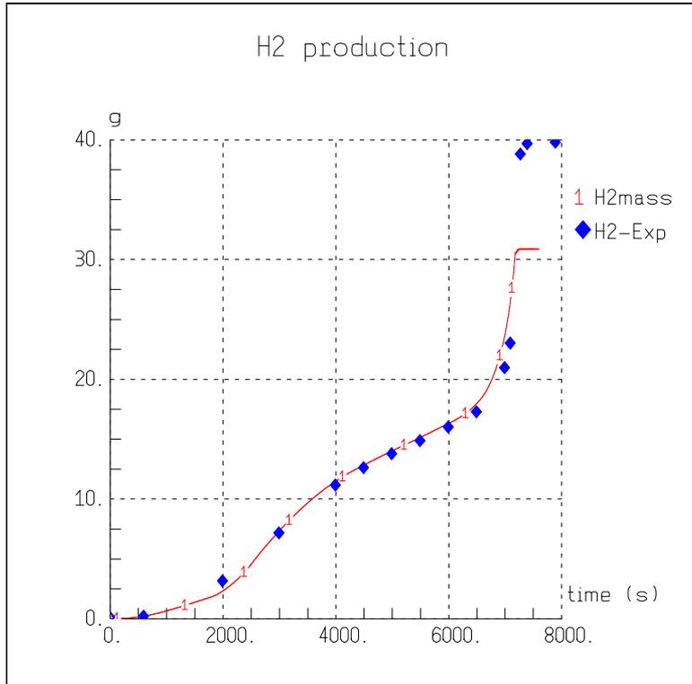
Fig.10 Hydrogen production – experimental & ASTEC
