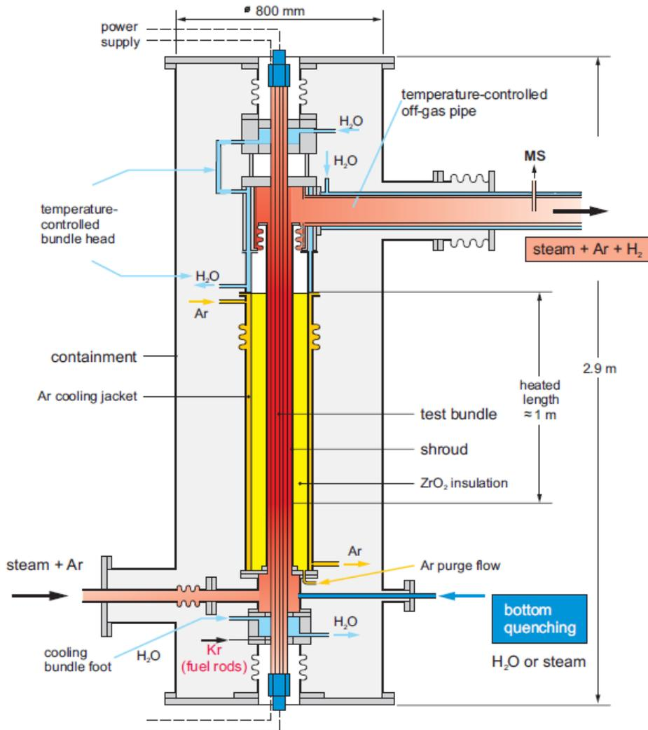
Fig.1 QUENCH-14 Test section
