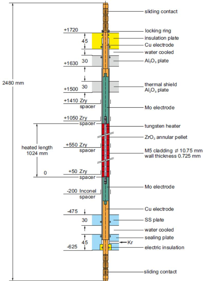
Fig.2 Fuel rod simulator
