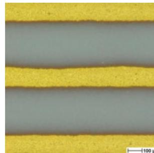
**BST films on an Au-electrode, sintered at 850°C**
