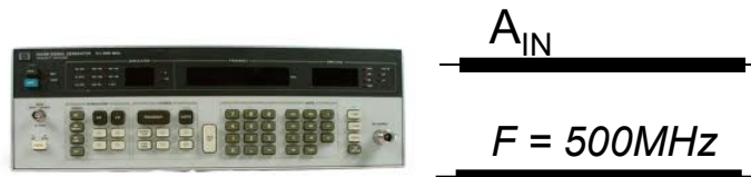
ADC characterization @ 500MHz square analog input
