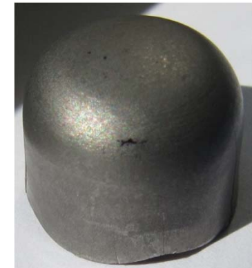
Ø28 mm sheet, 700°C, path-controlled ~1 µm/s
