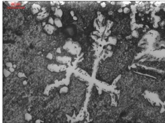
**Precipitations in adherent Pb-15.7Li scale**
