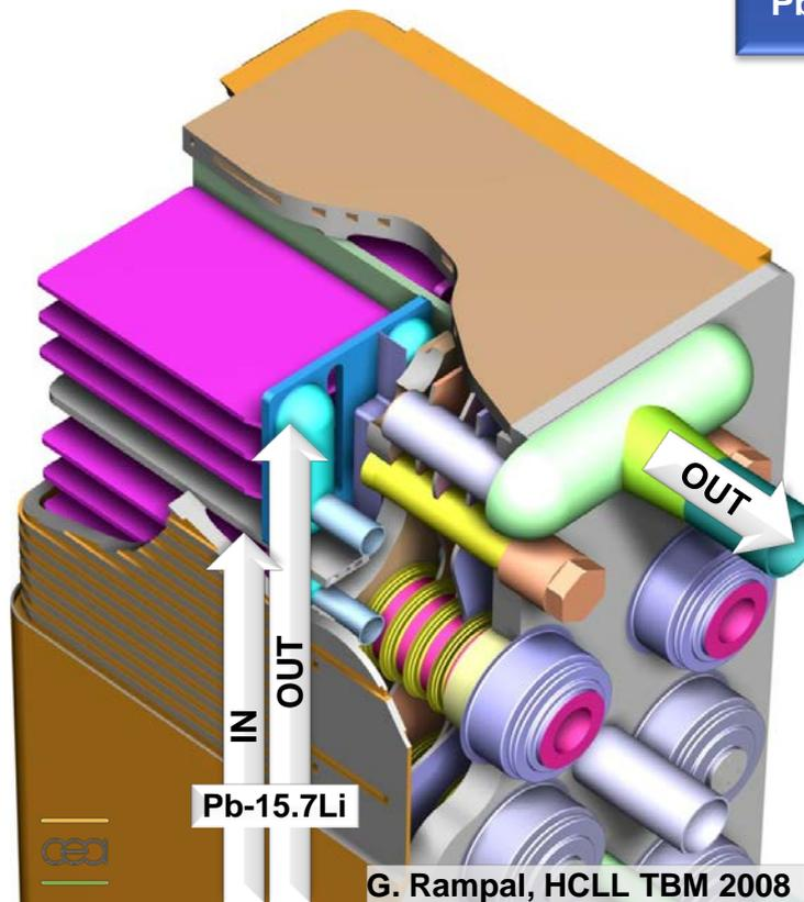
Corrosion of cooling and stiffening plates by PbLi and permeation of tritium from PbLi into He gas
