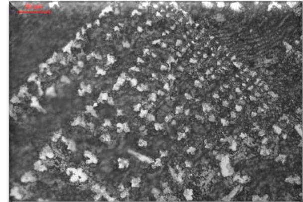
**Precipitations in the center of the magnetic trap parallel to field lines**
