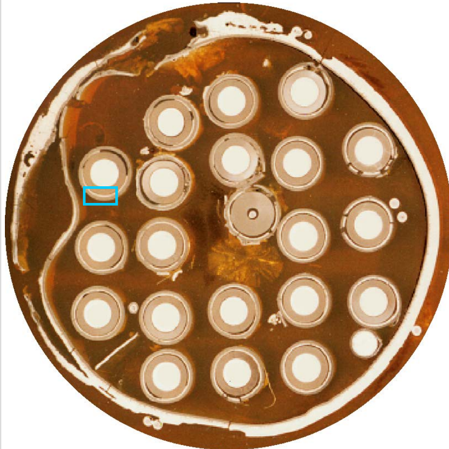
Q06: melting of cladding internal metal layer and shroud external metal layer
