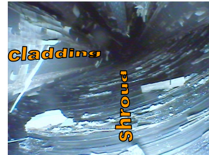
650 mm: spalled oxide scales at shroud and cladding
