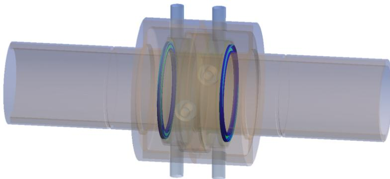
The maximum equivalent stress is in the nickel spacer rings and it amounts to **385 MPa**.
