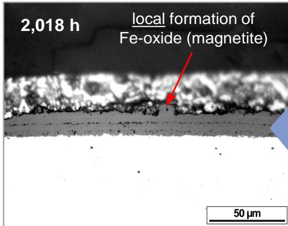
Cr-enrichment in oxide scale at metal/scale interface
