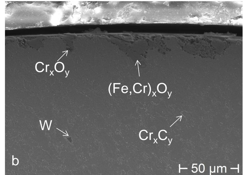
(b) cross-sections of the steel ruptured after  $t_R=2,982$  h in Pb at 329 MPa
