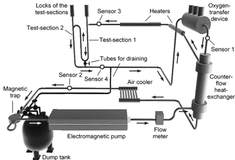
CORRIDA loop for materials testing in flowing oxygen-containing LBE
