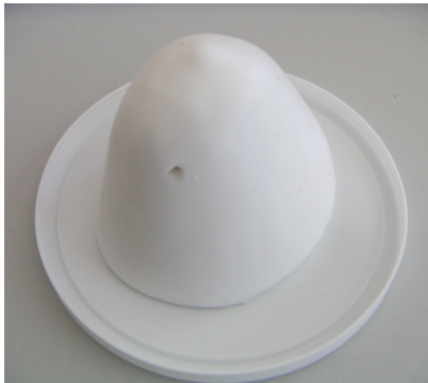
Figure : Triple Modality Breast Phantom (CIRS,USA)
